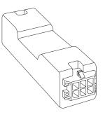
Connect this end to the CA6 Cable Assembly running to the first Primary Hub.
